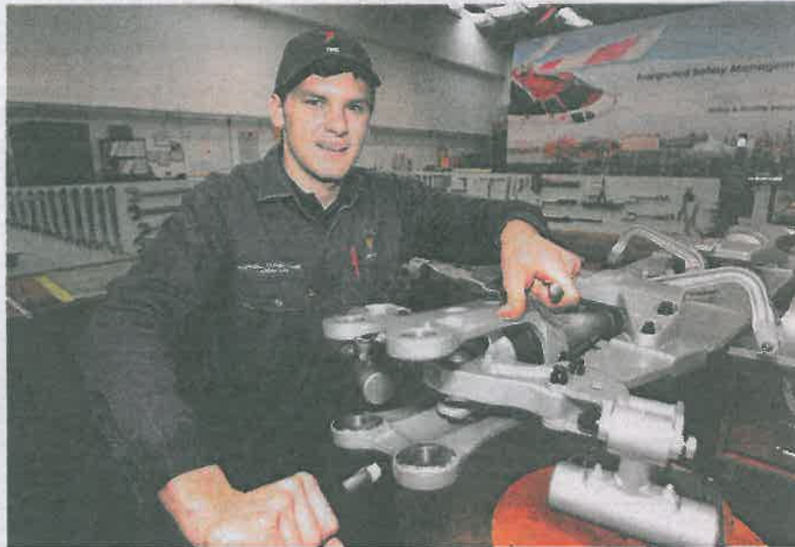
SECURE: Australian Technical College student Jarrod Jonker working on a main rotor hub for a Bell 412 helicopter at CHC Helicopters.
